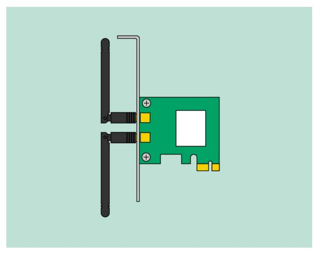
The **network card** allows your computer to communicate over a network and access the Internet. It can either connect with an **Ethernet** cable or through a **wireless** connection (often called **Wi-Fi**). Many motherboards have built-in network connections, and a network card can also be added to an expansion slot.
