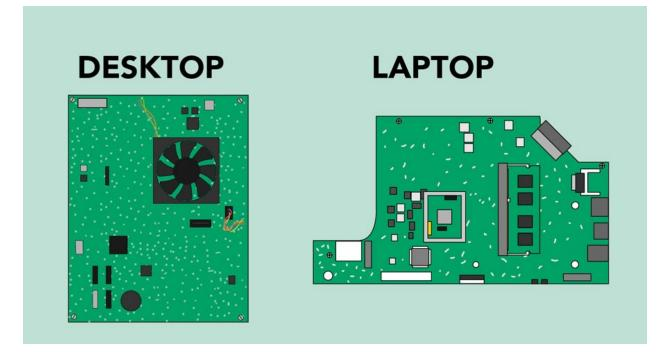
The **motherboard** is the computer's **main circuit board**. It's a thin plate that holds the CPU, memory, connectors for the hard drive and optical drives, expansion cards to control the video and audio, and connections to your computer's ports (such as USB ports). The motherboard connects directly or indirectly to every part of the computer.
