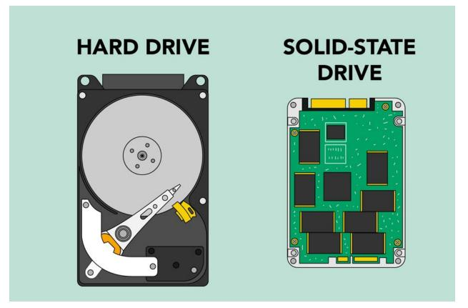
The **hard drive** is where your software, documents, and other files are stored. The hard drive is **long-term storage**, which means the data is still saved even if you turn the computer off or unplug it.
