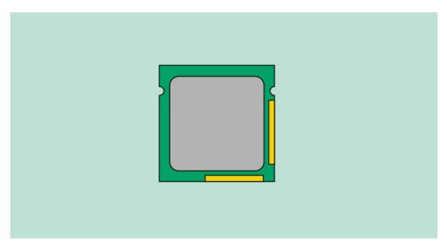
The central processing unit (CPU), also called a **processor**, is located inside the **computer case** on the motherboard. It is sometimes called the brain of the computer, and its job is to carry out commands. Whenever you press a key, click the mouse, or start an application, you're sending instructions to the CPU.
