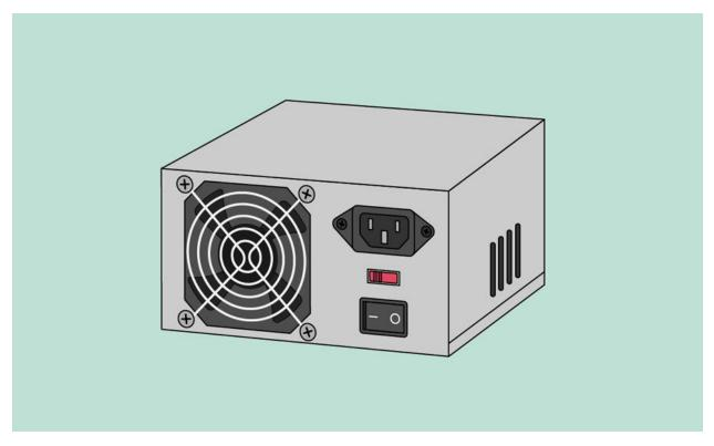
The power supply unit in a computer **converts the power** from the wall outlet to the type of power needed by the computer. It sends power through cables to the motherboard and other components.
